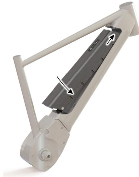
The BMZ E-Bike system can be combined with a number of different rechargeable battery variants. The assembly and removal of the rechargeable battery depends on the rechargeable battery model used. You can obtain detailed information about this from your cycle manufacturer and your bicycle dealer.
